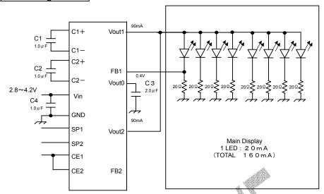
These figures are showing as the standard application example. The current values or so are considered whenever it is designed.
