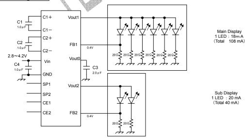
These figures are showing as the standard application example. The current values or so are considered whenever it is designed.
