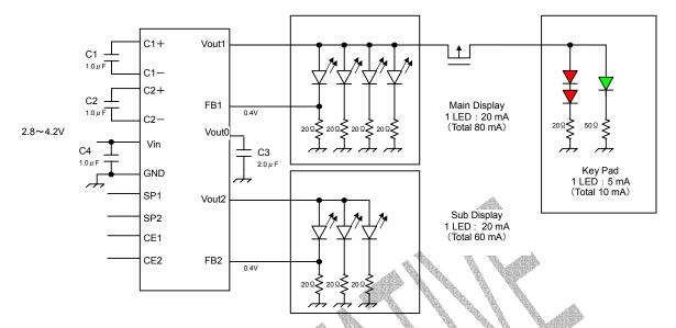
These figures are showing as the standard application example. The current values or so are considered whenever it is designed.
